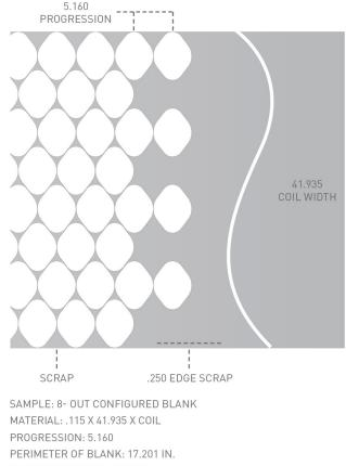
NET WT OF BLANK: .730 LBS. GROSS WT OF BLANK: .881 LBS
